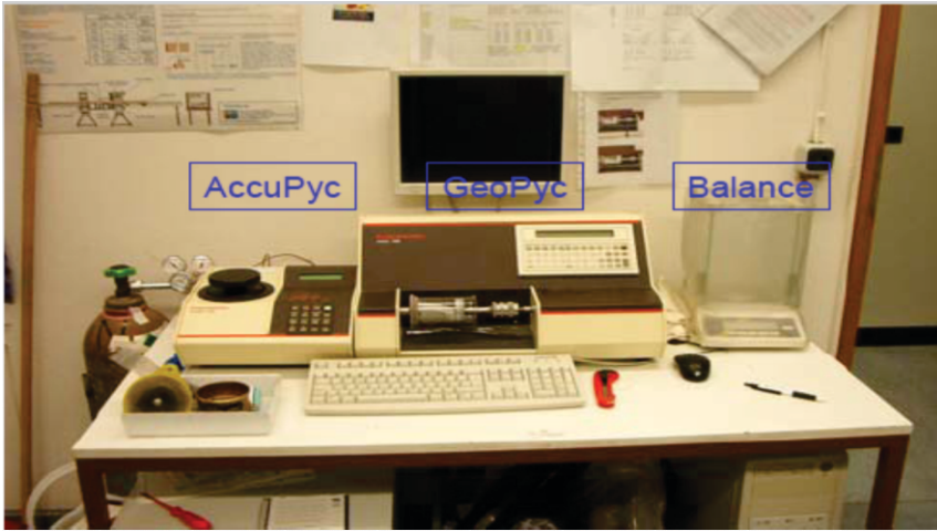
Figure 2: Array of the experimental design showing the Accupyc, Geopyc and weighing balance in array
